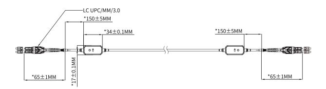
Tracking fiber optic jumpers are designed for (FTTH) intra-enterprise networks, and other fiber optic identification needs. Both ends of the tracking fiber optic jumper are assembled by conventional connectors (LC/SC/FC/ST), which contains a connector, a cover, a light-emitting device, a conductor, etc.
